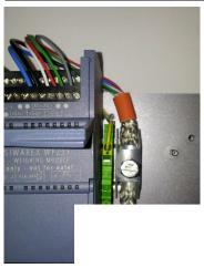
Important: The usage of a shield connector is highly recommended to avoid EMC interferences!
